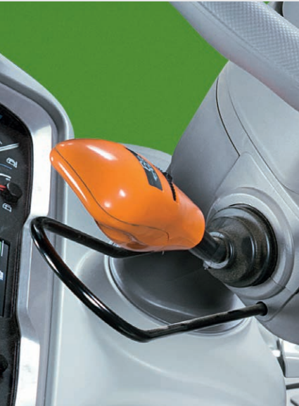
↑ Sense Clutch PowerShuttle.
